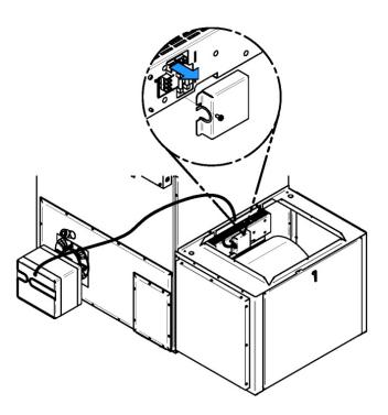
To facilitate connections, the use of a junction box is recommended. It can be installed on the back of the furnace. Use the following diagram for reference. Refer to the wiring diagram for complete connections.
