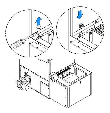
**Step 2.** Remove the screw that holds the power board cover which is found inside the blower box.
