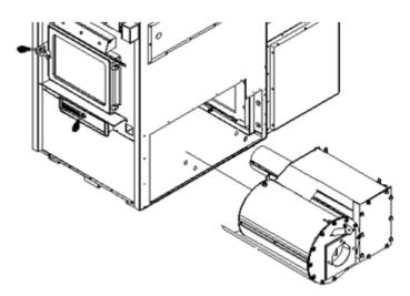
**Step 5.** Use the bolts on each side of the oil unit to have it leveled.
