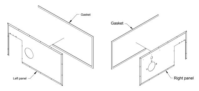
**Step 7.** Install the gasket on the oil unit combustion chamber cover. Then install the right panel from **Step 6** and the right electric element lid with the screws (22X) removed from **Step 1**.
