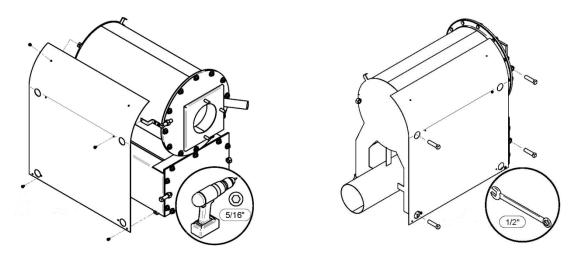
**Step 3.** Remove the view tube cap.
