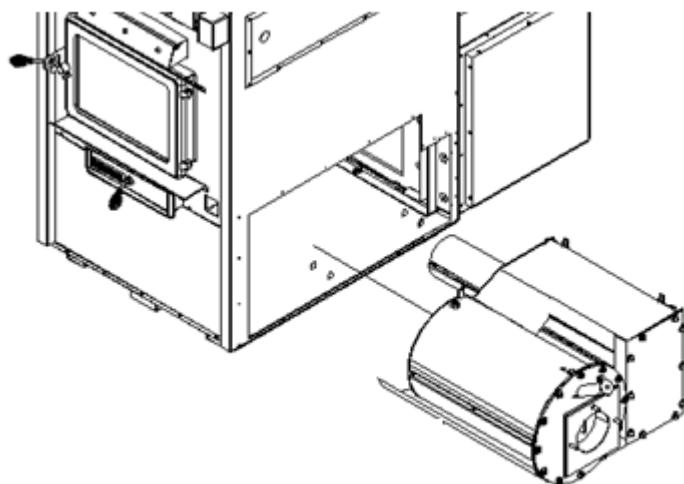
**Step 5.** Use the bolts on each side of the oil unit to have it leveled.
