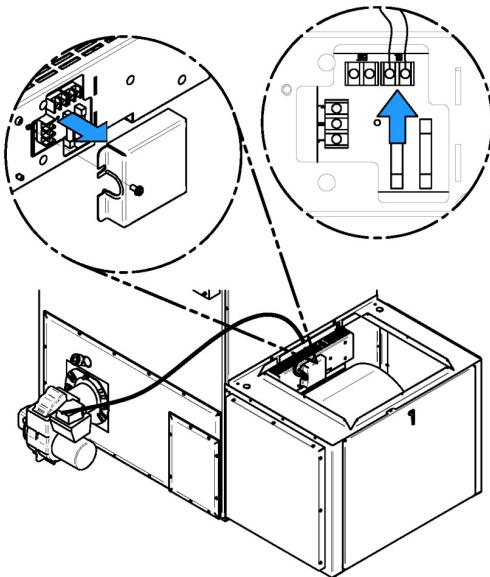
To facilitate connections, the use of a junction box is recommended. It can be installed on the back of the furnace. Use the following diagram for reference. Refer to the wiring diagram for complete connections.
