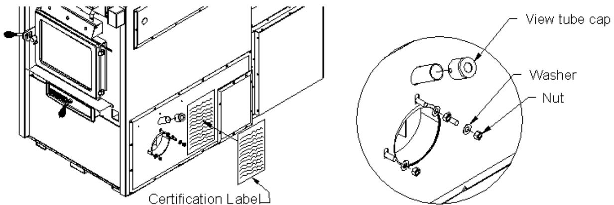
**Step 9.** Secure the left panel with the gasket installed in **Step 6** using the screws. Secure the left electric element lid back in place.
