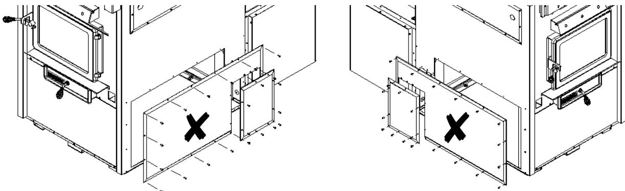
**Note:** To install the oil unit on the left side of the furnace, replace Step 2 by the Section “*additional steps for left side installation*”. Continue the installation from Step 3.
