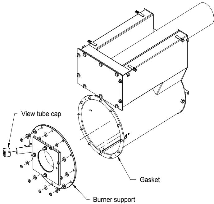
**Step 2.2:** Rotate 180 degrees the parts removed in **Step 2.1**. In order to do so, first install the gasket on the firebox of the oil unit. Then, secure the burner support onto the firebox using the nuts and washers. Remove the screws already secured to the firebox and use them to install the deflector support onto the firebox. Install the deflector and secure it in place using 4 screws. The screws and the deflector are supplied with the oil unit.
