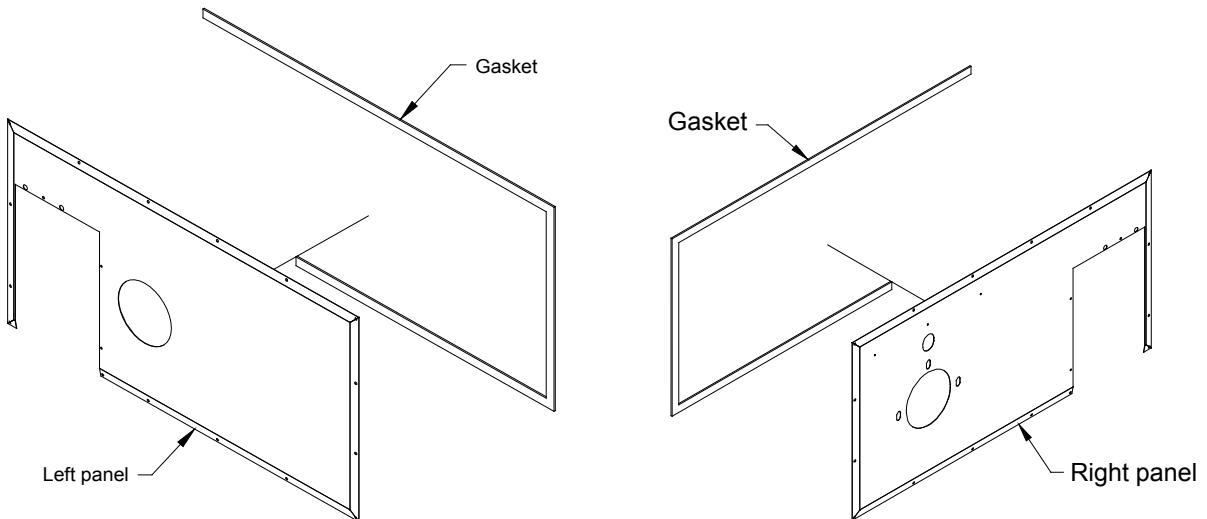
**Step 7.** Install the gasket on the oil unit combustion chamber cover. Then install the right panel from **Step 6** and the right electric element lid with the screws (22X) removed from **Step 1**.
