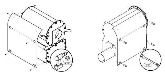
**Step 3.** Remove the view tube cap.
