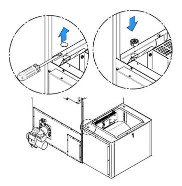
**Step 2.** Remove the screw that holds the power board cover which is found inside the blower box.
