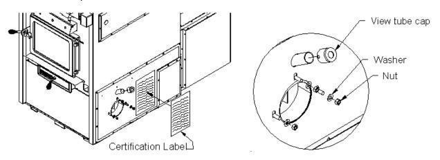
**Step 9.** Secure the left panel with the gasket installed in **Step 6** using the screws. Secure the left electric element lid back in place.
