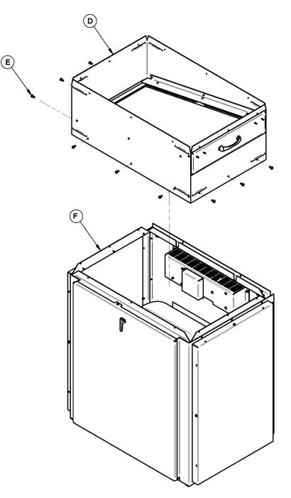
**Step 4**: Install the elevator bolts (H), provided with the user's manual, under the blower box assembly in the holes intended for this purpose. Secure the blower box (D) to the furnace with the screws (G) removed in **Step 2**. Level your blower box using the elevator bolts.
