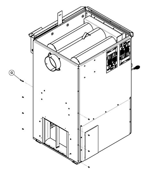
Step 2: Unscrew the eight screws (G) on the furnace, as shown. Keep.
