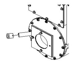
**Step 7.** Slide the oil unit **(R)** in the furnace.
