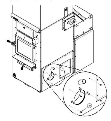
Step 14. Install the burner (AA). Secure it with washers (Y) (3X) and nuts (Z) (3X) (Beckett unit).
