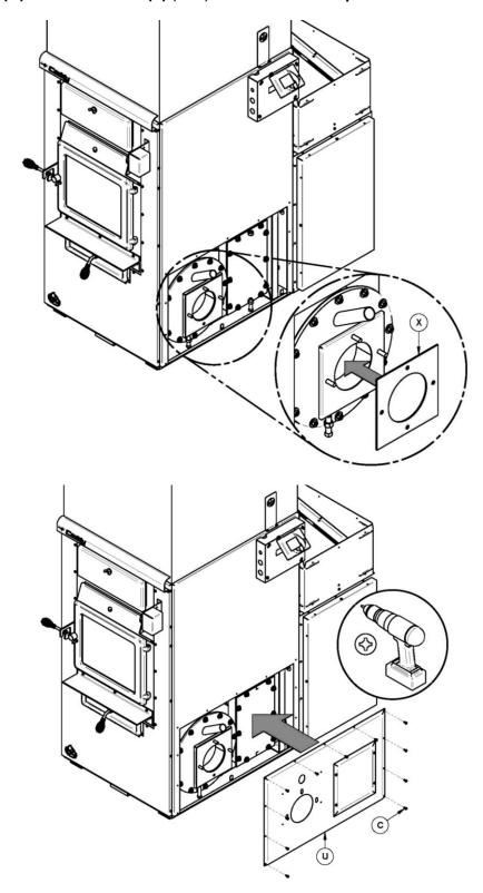
**Step 13.** Install 4 screws **(W)** on the right side panel to plug the holes.
