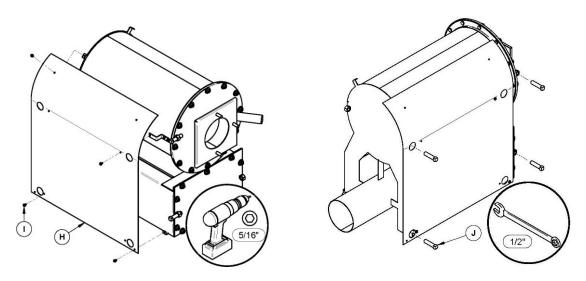
**Step 6.** Remove the vision tube cap.
