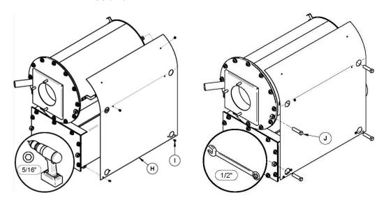
Step 5.4: Secure air jacket panels (V) (2X) using screws (W) (4X) on both panels (S) and (U).
