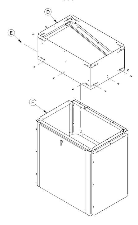
**Step 4**: Install the elevator bolts (H), provided with the assembly, under the blower box assembly in the holes intended for this purpose. Secure the blower box (D) to the furnace with the screws (G) removed in **Step 2**. Level your blower box using the elevator bolts.
