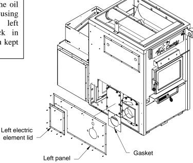
Step 9: Put the view tube cap back in place (it was removed in Step 1). Install the oil unit using nuts and washers supplied with the option as shown on the right. It is important to stick the certification label next to the unit.
