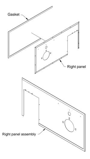
Step 7: Before installing the right panel, put the gasket on the oil unit. Secure the right panel using the screws. Secure the right electric element lid back in place using the screws you kept from Step 3.
