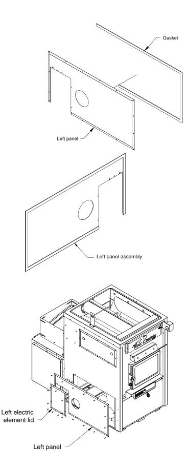
Step 10: Secure the left panel using the screws. Secure the left electric element lid back in place using the screws that you kept from Step 4.
