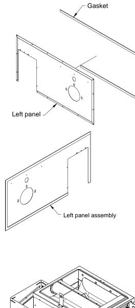
Step 8: Before installing the left panel, put the gasket on the oil unit. Secure the left panel using the screws. Secure the left electric element lid back in place using the screws you kept from Step 4.
