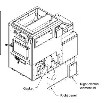
Step 8: Put the view tube cap back in place. Install the oil unit using nuts and washers supplied with the option as shown on the right. It is important to stick the certification label next to the unit.
